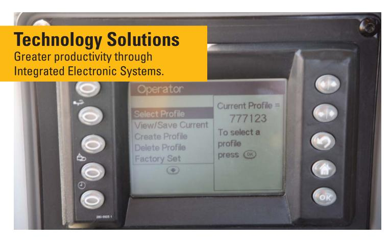
The 994H electronic systems have been completely integrated to function as one machine. This integration creates a smart machine and more informed operator, maximizing the productivity of both.
