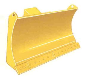
Power Angling and Tilt 3P Dozer makes it easy to grade, backfill ditches, landscape or spread fill. You can angle it 25° left or right. Tilt it 8-1/2°. All with two simple controls. One lever controls raise, lower and tilt. The other lever angles the blade left or right. Large capacity enhances productivity in spreading and backfilling applications.
