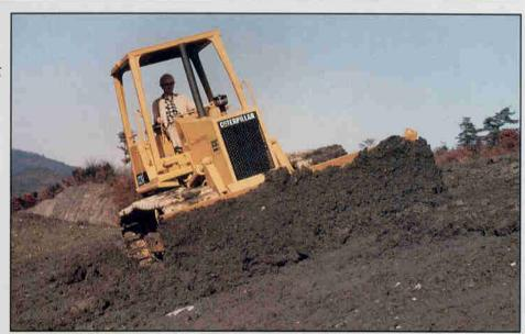
Self-cleaning shoes, 635 mm/ 25", available for improved performance in cohesive material and reduced build-up between shoes.
