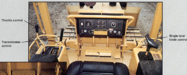
Walk through operator's compartment
