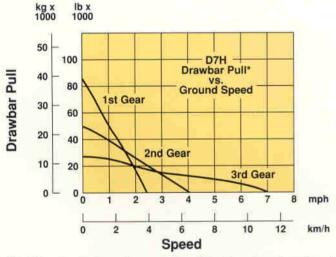
\*Usable pull will depend on weight and traction of equipped tractor.
