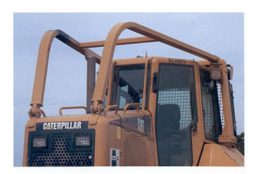
Forestry Sweeps. In forestry and land clearing applications where limbs and debris can damage a machine, optional sweeps are available for the N-Series. Sweeps help to shield critical components on the tractor such as hydraulic lines, exhaust stacks, cab windows and lights from damage. Rear Counterweight. Rear counterweights are available and can be used to help the machines balance in severe applications such as backing up slopes or heavy angle dozing.
