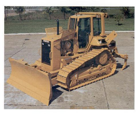
Built-in Serviceability. Less service time means more working time. Major components are designed as modules and most can be removed without disturbing or removing other components.
