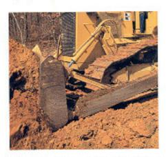
Semi-Universal Blade (XL Arrangement Only). Built for tough applications where penetration and blade side loading are important. The design of the SU blade makes it excellent for aggressive dirt penetration and loading materials. The blade wings are designed for superior load retention.
