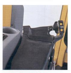
Finger Tip Control (FTC). Located to the operator's left, finger tip controls provide one-handed operation. They control steering, machine direction and gear selection.
