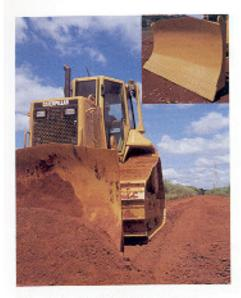
Caterpillar Blades, With superior moldboard and 4-cell structure design, Cat hulldozer blades hold up to the toughest job conditions. Our high-tensile strength blades resist torsional bending and deflection in tough applications.
