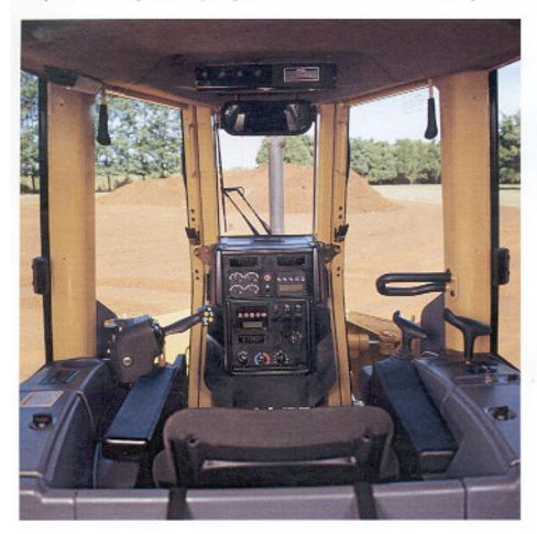
Cab. The cab incorporates large glass window and door panels. This allows for excellent visibility to the blade, rear and sides of the machine. New door and window seal design allows for a fully pressurized dust free cab. Low acoustic headliner material, and sound suppression foam panels reduce sound levels to below 76 dB(A) when measured per ISO 6394:1998.
