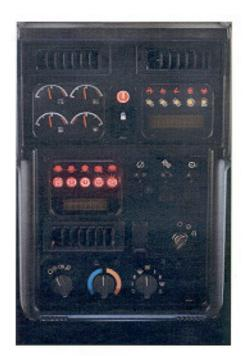
Dash. The instrument panel, with easy to read analog gauges and warning lamps, keeps the operator aware of any potential problems. All gauges and readouts are easily visible in direct sunlight. HVAC controls and vents are conveniently located on the dash to provide climate control for the operator. Auto-shift and Auto-kickdown controls are located within easy reach of the operator. New footpads keep the operator stable and comfortable during side slope applications.
