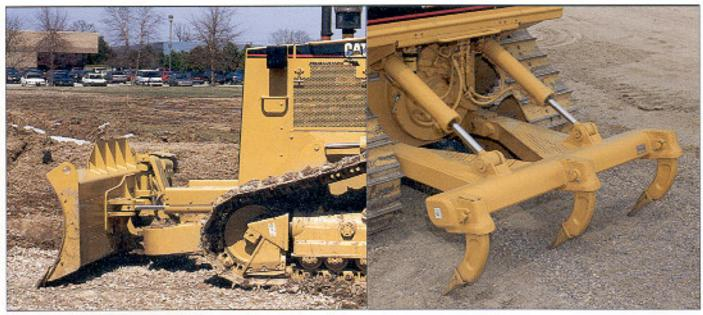
Variable Pitch Power Angle and Tilt (VPAT) Blade. Manually adjustable blade pitch for optimum performance.
