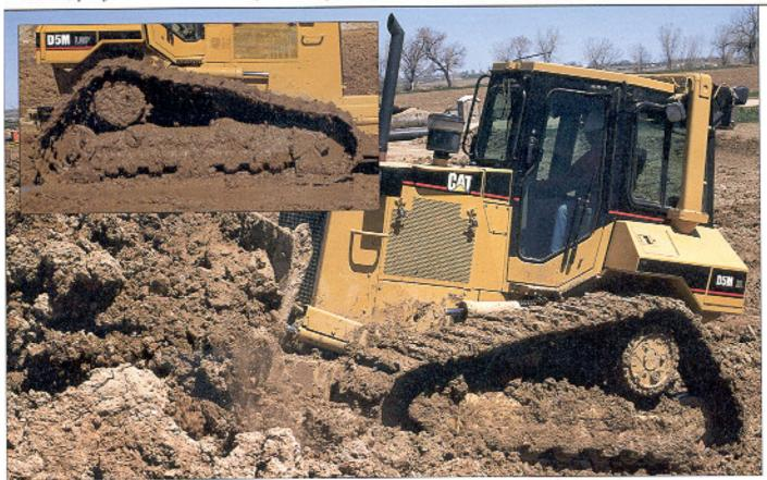
Final drives and associated power train components are raised above the work area, isolating them from groundinduced impact loads, as well as implement and roller frame alignment loads, extending power train component life.
