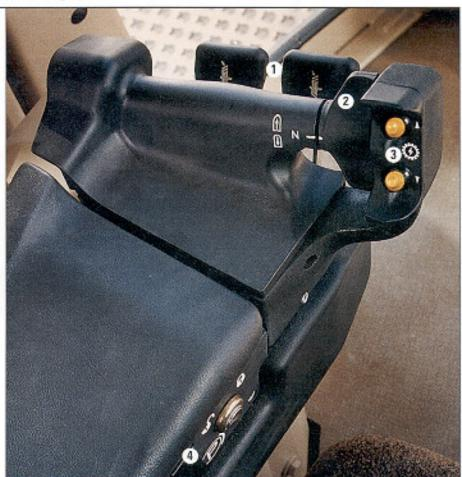
3 Gear selection is made by two buttons to the right of the machine direction knob. The top (up-shift) button shifts the machine transmission to the next higher gear while the bottom (down-shift) button shifts to the next lower gear.
