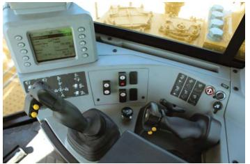
The Finger Tip Controls (FTC) require less effort and are more comfortable for long periods of operation. Single-hand controls located on the left armrest coordinate steering using left and right finger paddles located ahead of the handgrip. The D11T/D11T CD uses electro-hydraulic clutch-brake steering.
