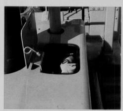
**ROUTINE MAINTENANCE** and fluid level checks are convenient. Air cleaner: engine oil filter, fill port and dipstick; radiator fill; hydraulic reservoir; fuel tank and strainer—all are easily accessible.
