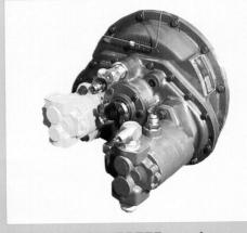
TORQUE CONVERTER transfers power smoothly from the engine to the transmission. Keeps torque up, absorbs shocks and matches track speed to hydraulic power.
