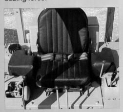
operator efficiency is virtually assured by a functionally designed compartment that features an adjustable seat, conveniently located controls, and strategically grouped gauges. A suspension seat, adjustable to the operator's weight, is optional.
