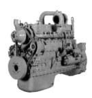
Komatsu S6D110 turbocharged diesel engine — offers hig power and maximum fuel economy. This engine delivers a powerful 140 FHP at 2500 RPM, and its high torque rise makes even the toughest digging easy. A direct-injection fuel system contributes to reduced fuel consumption.
