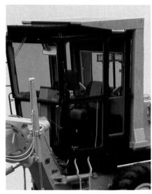
Rear mounted, sound suppressed cab — provides excellent visibility and plenty of work space. Insead of the conventional unitized ROPS cab, theGD615A is equipped with a separate cab and externallymounted ROPS. This enables slim cab pillars and means plenty of interior cab space and improved overall vision. Tinted glass windows reduce glare and keep the cab cooler in hot weather. The front window can be swung up and out of the way for unimpeded forward visibility.
