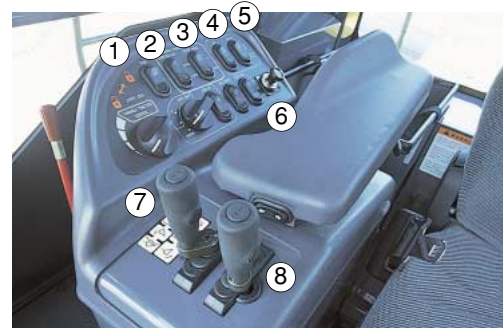
1:ECSS 2:Remote Boom positioner switch 3:Remote bucket digging angle control switch 4:RPM set (On/Off) (option) 5:RPM idle set (option) 6:Semi-auto digging system (option) 7:Boom control 8:Bucket control
