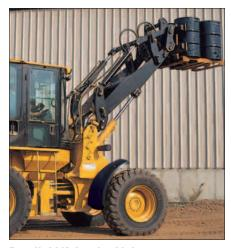
Parallel Lift Loader Linkage. The IT28G's 8-bar parallel design linkage keeps work tools such as forks level throughout the range of lift without adjustment by the operator. Superior load control is provided by more tilt capacity than lift in all positions. Long lift arms, tall front tower and high pivot points offer more height and reach than conventional loaders.
