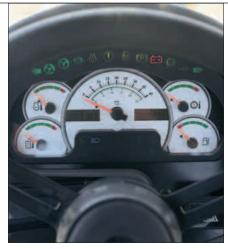
**Instrument Panel.** Redesigned instrument panel is conveniently located with easy-to-read gauges and expanded warning/indicator and diagnostic functions.
