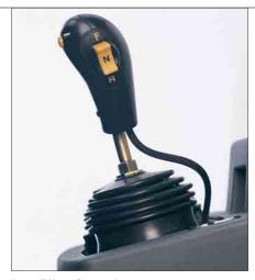
**Low Effort Operation.** Joystick hydraulic controls provide ease of lift and tilt functions. A single joystick is standard. An integrated directional control switch on the joystick provides easy operation and enhanced productivity. A two lever control is optional.
