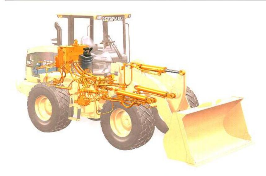
Modular hydraulic system designed by Caterpillar provides low-effort operation and greater control:
