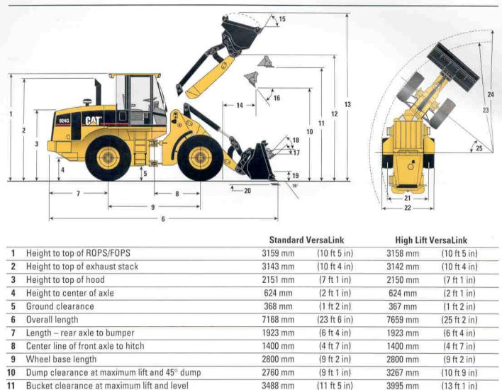
Dimensions listed are for machines equipped with 17.5-25 12PR (L-2) tires and 1.8 m³ (2.3 yd³) general purpose bucket with bolt-on cutting edge. Refer to Operating Specifications for bucket variations.
