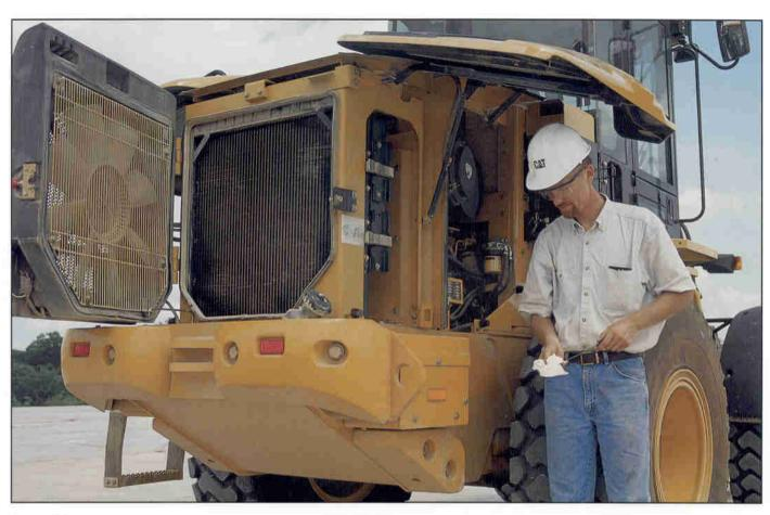
Easy, wide open access. Gull-wing doors with pneumatically-assisted lift cylinders effortlessly lift up for exceptional access to the engine and power train components. All filters and service points are within easy reach.
