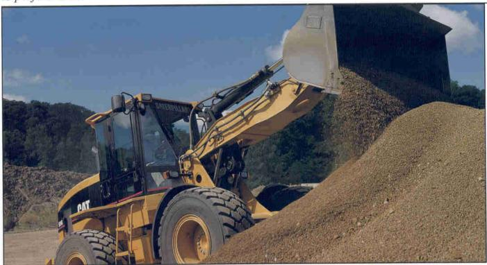
The 924G uses a revolutionary new design - VersaLink Loader Linkage (patented), a one-piece fabricated box-section lift arm.
