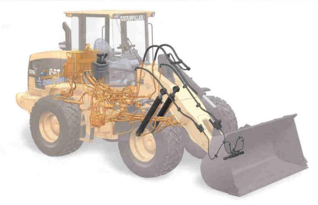
**Modular hydraulic system** designed by Caterpillar provides low-effort operation and greater control:
