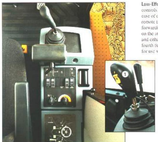
Low-Effort Operation. New pilot hydraulic controls give the 914G uncompromised ease of operation of lift and tilt functions. A remote transmission control option adds a forward/neutral/reverse control switch (1) on the implement lever for easier operation and enhanced productivity. Third and fourth function controls are also available for use with special attachments.
