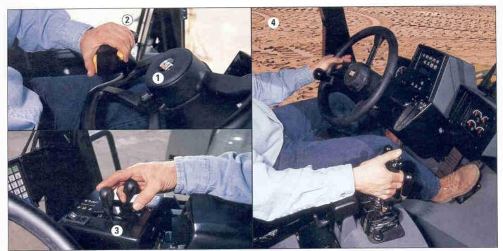
The 950G is available with two different configurations of operator controls – one with electro-hydraulic implement controls and Command Control steering, and another with pilot hydraulic implement controls and Conventional steering. Customers who want the ultimate in operator comfort and efficiency have a choice.
