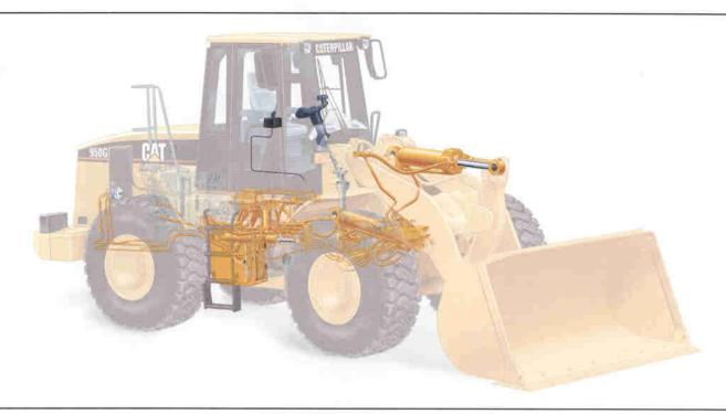
**Low-effort hydraulic controls** allow the operator to precisely maneuver bucket lift and tilt.
