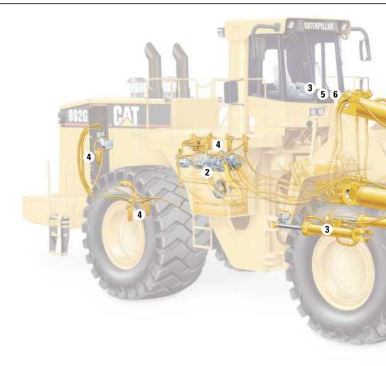
3 Load Sensing Steering with STIC control system integrates steering and transmission into a single controller. The steering system utilizes a variable displacement pump for maximum machine performance by directing power through the steering system only when needed.
