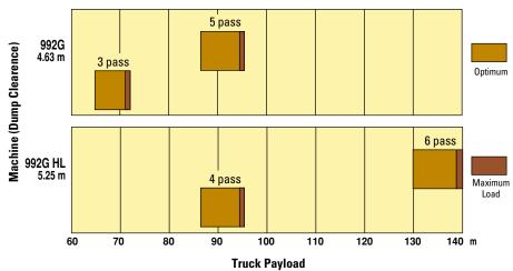
777D = 92 Metric Tons maximum payload 785C = 146.1 Metric Tons maximum payload
