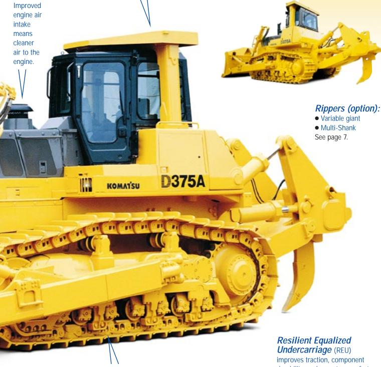
Low-drive, long-track, seven roller undercarriage ensures outstanding grading ability and stability.
