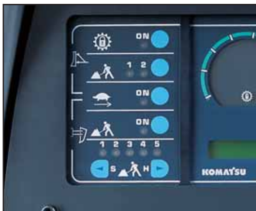
Track shoe slip control panel
