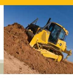
No need to cross-steer or ride a brake. These dozers steer the same and maintain their preset speed whether working on level ground or a 2-to-1 slope.
