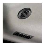
Automotive-style directional vents deliver effective airflow to keep the glass clear and the cab comfortable. Air conditioning is standard on all cabs. For ROPS-only crawlers, an optional underseat heater helps warm the operator.
