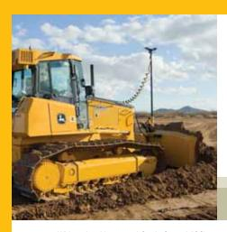
With optional Integrated Grade Control (IGC), your dozer arrives from the factory "plug and play" ready. Its open architecture design lets you employ the electronic grade-control system that's right for you.
