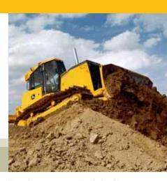
No need to cross-steer or ride a brake with these dozers. The 750J and 850J steer the same and maintain their preset speed whether working on level terrain or a 2-to-1 slope.
