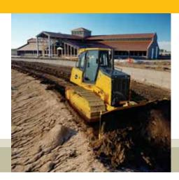
Independent track control lets an operator speed up or slow down each side, for smooth, full-power turns. An automatic 10-percent horsepower boost helps carry more material in a turn.
