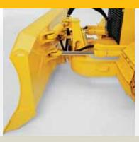
The PAT dozer's closedcell blade design and box-section C-frame deliver exceptional strength and durability. Outside-mounted dozer push beams are equally durable.
