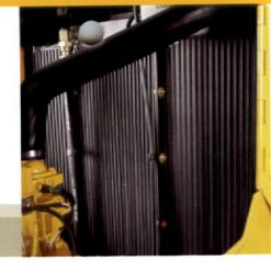
No stacked coolers in these crawlers. Side-by-side cores with wide fin spacing reduce clogging and are easy to clean.
