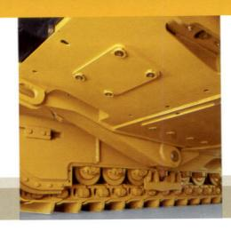
Unitized mainframe with flush-fit bottom guards combines with tight-fitting side shields to prevent debris from being drawn into the engine compartment.
