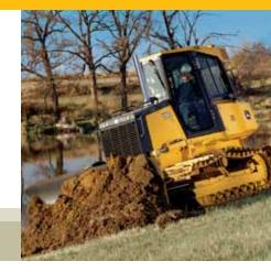
The 700J steers the same and maintains its preset speed whether it's on level ground or a 2-to-1 slope. For total control regardless of the terrain.
