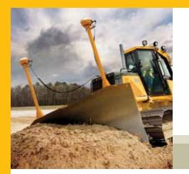
Equipped with optional Intergrated Grade Control (IGC) package, your dozer arrives from the factory "plug and play" ready. Open architecture design lets you employ the electronic grade control system that's right for you.
