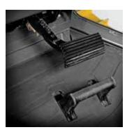
Choose the decelerator function that's right for the job. Slow both ground speed and engine rpm, or ground speed only to help maintain traction without affecting engine power and hydraulic response. Fully depressing the pedal applies the brakes.
