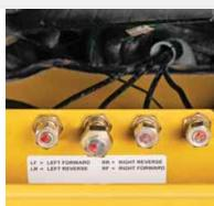
Remote test ports and diagnostic messaging enable technicians to quickly troubleshoot problems.
