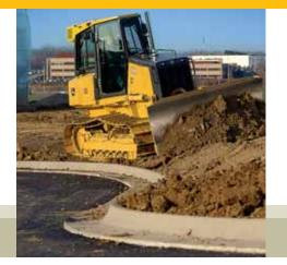
Infinitely variable track control lets you speed up or slow power to either track, delivering smooth, full-power turns that don't rob horsepower or tear up soft terrain.
