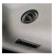
Automotive-style directional vents help keep the view clear, while delivering warm or cool air quietly and efficiently. Air conditioning is standard on all cabs. An optional under-seat heater is available for non-cab crawlers.
