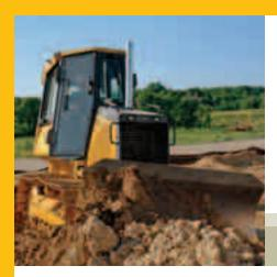
Counterrotation is a productivity-boosting feature that enables the operator to overcome heavy corner loads and to quickly reposition the blade on the go. Provides space-saving spot turns, too.
