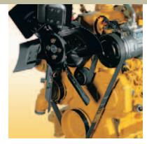
Serpentine belt never needs adjusting. 500-hour service interval lets you go longer between engine oil changes.
