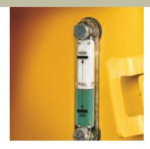
Conveniently located easyto-read sight gauge lets you check hydraulic-fluid levels at a glance.
