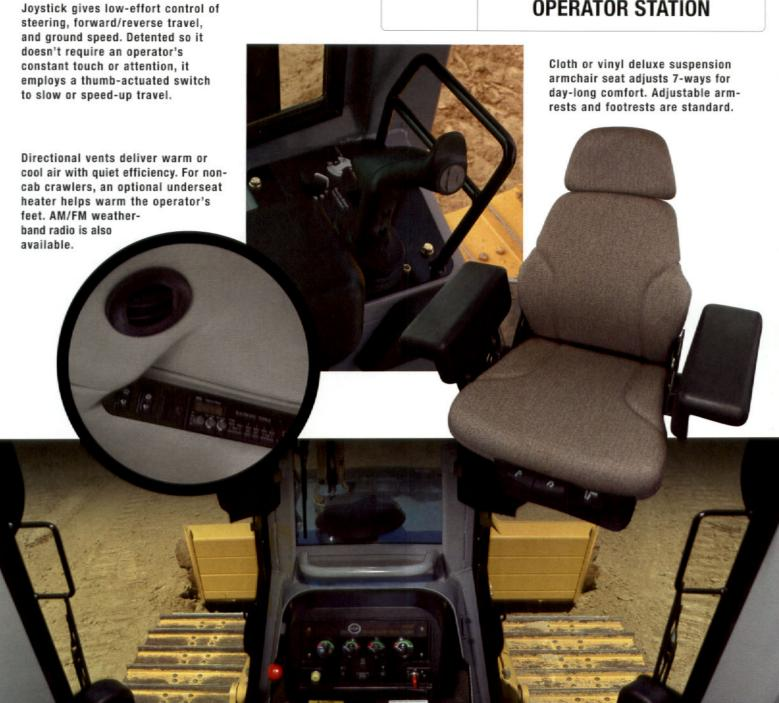
Operators won't have to feel their way on a 700H. Its cab-forward design and floor-to-ceiling tinted glass provide a commanding view.
