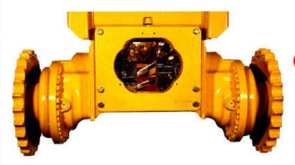
Axial-piston hydrostatic motors are mounted directly to the final drives at the back of the mainframe. A rear access panel makes removal easy. Heavy-duty high-pressure hoses connect the pumps and motors that form the drivetrain. O-ring face seal (ORFS) couplings virtually eliminate leaks.
