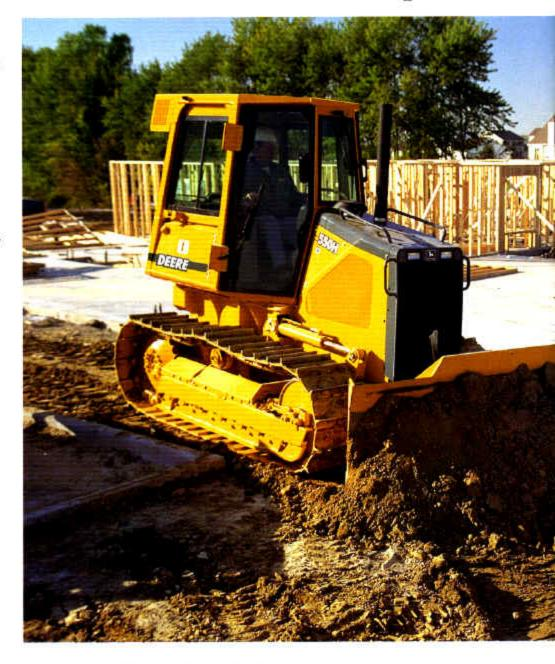
Functional counterrotation is another distinct Deere advantage. It's especially helpful for overcoming corner-loaded side-drafts and for quickly repositioning the blade on-thego. Or use it for space-saving spot turns, no matter what's underfoot.
