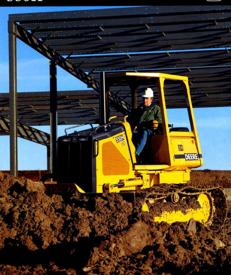
Power management system takes both the guess and work out of efficient operation. Just set the ground speed lever to the maximum desired speed and the dozer does the rest. As loads change, the drivetrain responds, automatically powering up or down to maintain peak engine rpm and efficiency without stalling. Perhaps best of all, it's fully functional at any engine speed.
