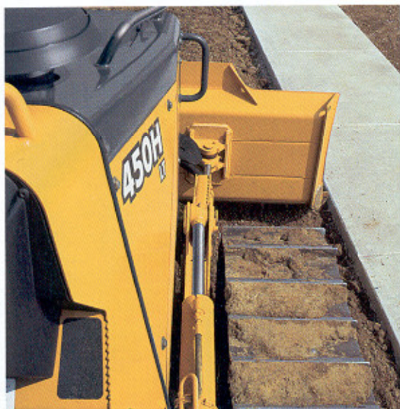
What a view! The narrow dash, tapered sheet-metal, small-diameter front idlers, center-section spillsheet, high blade heel, and angled blade end plates all contribute to unsurpassed visibility, with or without cab.
