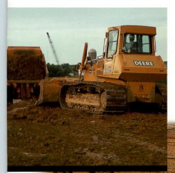
Power management system takes both the guess and work out of efficient operation. Just set the maximum desired ground speed and the dozer does the rest. As loads change, the drivetrain responds, automatically powering up or down to maintain peak engine rpm and efficiency.
