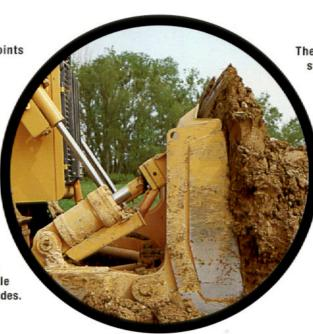
The semi-U dozer's tall spill sheet, steep curvature, and angled ends let this blade build and carry large loads. Quick-drop valve allows rapid blade repositioning.
