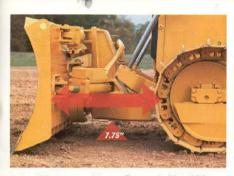
Angle cylinders are powerful, responsive, and positioned out of the dirt and where they resist dirt buildup.
