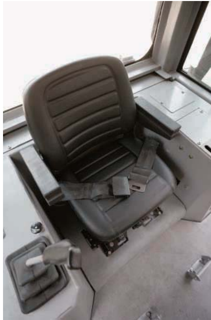
Seat. A comfortable suspension seat is able to be adjusted fore and aft for greater operator comfort. Arm rests also help provide comfort for all day operation. Wide 76 mm (3 in) seat belt is standard.
