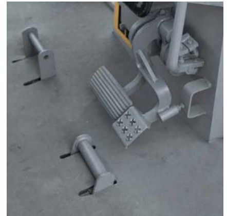
Brake Pedal. A single brake pedal actuates both tracks to make operation easier.
