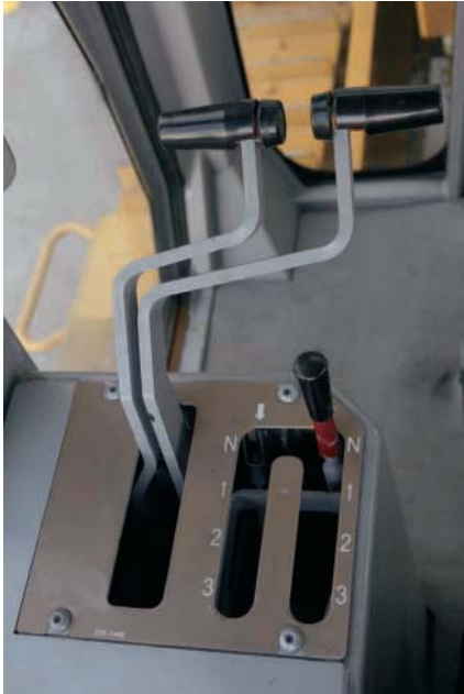
Directional Controls. Steering and transmission controls are located conveniently to the operator's left for comfortable operation.
