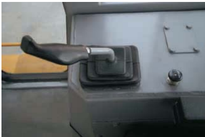
Dozer Blade Controls. The dozer controls are located on the operator's right hand side.
