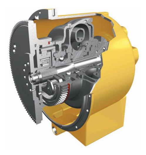
**Torque Divider.** An improved single-stage torque converter sends 70% of engine torque through a converter and 30% through a direct drive shaft for greater driveline efficiency and higher torque multiplication. The torque divider provides improved efficiency and broader range of performance in second gear dozing and scraper pushloading.
