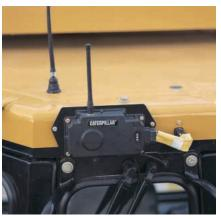
Product Link. The optional Product Link system is factory installed or easily retrofitted wireless system that simplifies equipment fleet tracking. Using satellite or cellular technology, the system automatically reports key machine parameters such as location, machine hours, active and logged service codes and security alarms. Depending on the Product Link version, it can connect with other on-board systems, issue e-mail or pager alerts and provide fuel consumption data.
