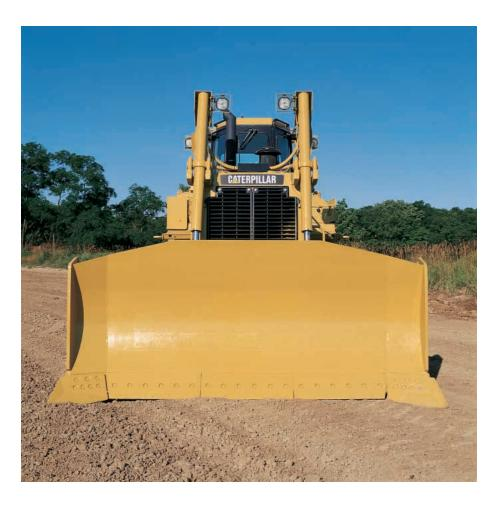
**Dozers.** With moldboard construction and hardened bolt-on cutting edges, Caterpillar bulldozer blades load easily and are durable. In tough applications, Caterpillar blades resist torsional bending and distortion thanks to their high-tensile strength.
