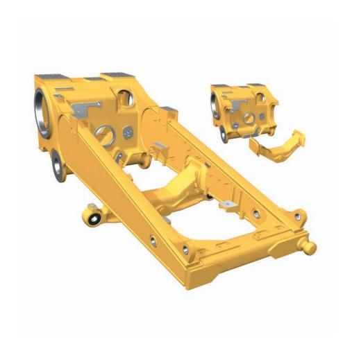
**Frame And Castings.** The D7R Series 2 frame is built to absorb high impact shock loads and twisting forces. Castings provide added strength to the main case and equalizer bar saddle.
