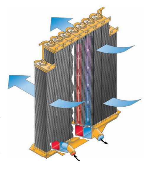
**Protection From Leaks.** To reduce the potential for coolant leaks, brass tubes are welded to a large, thick header, improving strength of the tube-to-header joint. In conditions where abrasive materials can be airborne, the attachment sand blast grid should be used to prevent core damage.
