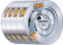
**Transmission.** The D7R Series 2 planetary power shift transmission features three speeds forward and three speeds reverse and utilizes large diameter, high-capacity, oil cooled clutches. To maximize the life of the transmission the planetary design distributes loads and stresses over multiple gears.
