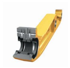
**Equalizer Bar.** The pinned equalizer bar gives the roller frames the ability to oscillate up or down to better match ground contours while providing maximum traction and operator comfort. Equalizer bar end pins are oil filled with limited slip seals for longer life and reduced repair costs.
