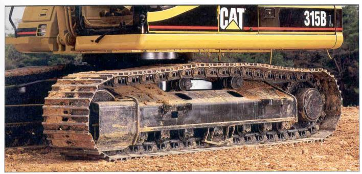
Precision robotic welding helps ensure quality welds. These welds increase rigidity, reduce internal stresses and enhance durability for the chassis and track roller frames.
