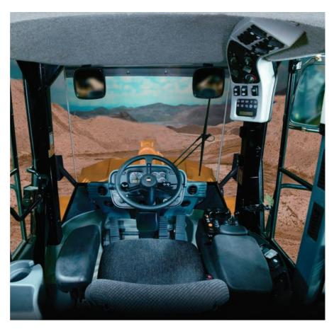
The Command Control Steering wheel contains the forward/neutral/reverse switch and the upshift/downshift button – allowing the left hand to remain on the steering wheel at all times. Implement controls are integrated into the right armrest so they move with the operator.
