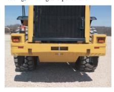
**Counterweight.** The one-piece counterweight is integrated into the 972H design and styling. This 5,849 lb (2653 kg) counterweight incorporates the rear lights into the top of the structure.
