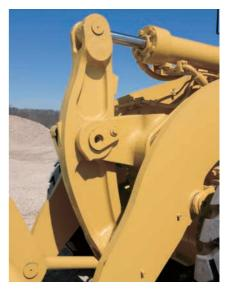
**Linkage.** The 972H linkage is a single-tilt Z-bar design. Z-bar linkage generates excellent breakout force and good rack back angle for better bucket loading and load retention.
