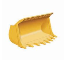
**Rock Buckets.** Rock buckets are designed for face or bank loading in mining or quarry applications. The straight-edge rock bucket provides higher breakout force and increased dump clearance. The spade-edge rock bucket offers increased penetration in certain applications.
