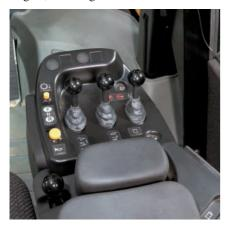
**Seat.** The Cat C-500 Series Comfort air suspension seat, standard in the 972H, is built strong and durable and is 6-way adjustable to accommodate all-sized operators. The cast one-piece back and seat pan prevent protrusions under the cushions. The seat features an automotive-style lumbar support for maximum comfort. The right hand armrest with integrated implement controls adjusts for comfortable, convenient operation. A heated seat option is available for additional comfort.
