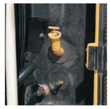
With the hood closed, quick checks of engine oil levels and the coolant sight gauge can be completed through the side service doors.
