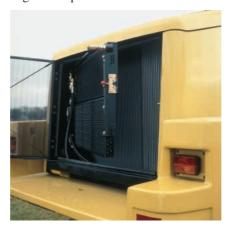
**COOLING SYSTEM.** Cooling system access for clean-out and maintenance is outstanding. The perforated and corrugated grill minimizes debris build-up and swings out for easy cleaning and access to the cooling cores.
