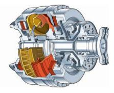
**5 Impeller Clutch.** Modulates the amount of engine power sent to the wheels.
