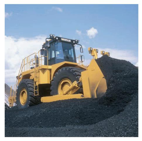
**Heavy-Duty Semi-U Blade**. Has the same configuration as the Semi-U blade but is built with thicker plates for more severe applications.
