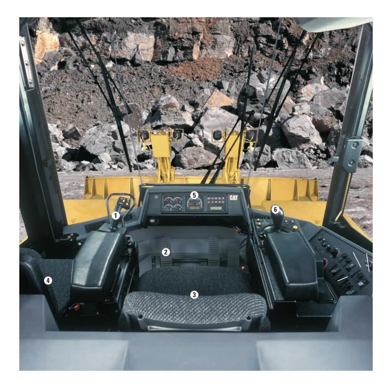
**Cab Design.** Is spacious and incorporates innovations for operator comfort and productivity, including an excellent viewing area, interior sound levels below 75 dB(A), Cat Comfort Series seat, standard coat hook, cup holder, storage bin, sun visor, trainer's seat with lapbelt and intermittent wet-arm wipers. It is also radio-ready for two-way radios.
