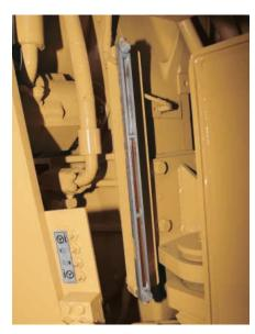
• **Sight Gauges.** In the hydraulic tanks, transmission and radiator provide quick check for fluid levels.
