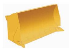
**Semi-U Blade.** Combines the characteristics of the S and U blades into one package. Provides increased capacity with the addition of short wings which include only the dozer end bits without sacrificing spreading characteristics of straight blades.
