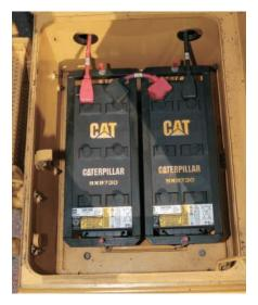
• **Batteries.** Are accessible through hinged doors in bumper.
