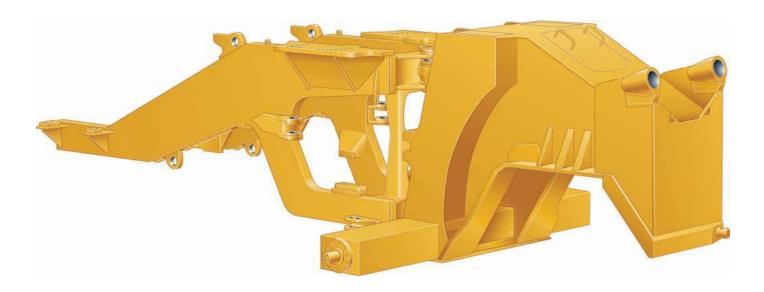
**Structure Welds.** Are more than 90 percent robotically welded. This provides highly consistent welds with deep plate penetration and excellent plate fusion. The benefit is greater fatigue strength and longer life than with conventional welding methods.
