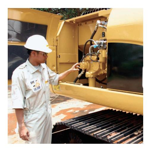
**Ground Level Service.** The design and layout of the 320D was made with the service technician in mind. Many service locations are easily accessible at ground level allowing critical maintenance to get done quickly and efficiently. **Air Filter Compartment.** The air filter features a double-element construction for superior cleaning efficiency. When the air cleaner plugs, a warning is displayed on the monitor screen inside the cab.
