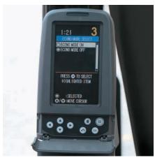
**Monitor.** The monitor is a full color 400x234 pixels Liquid Crystal Display (LCD) graphic display. The monitor angle can be adjusted to minimize sun glare and has the capability of displaying information in Indonesian and twenty-six other languages.
