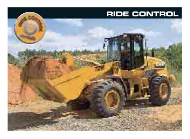
The ergonomically designed Case wheel loaders can be specified with Ride Control, a system that allows the lift arms to float when the machine is moving, preventing bounce in the cab and at the wheels. Ride Control allows the operator to drive at higher speeds during load and carry operations, offering excellent load retention and reducing fatigue for the operator.
