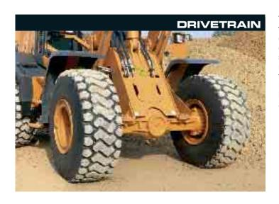
The 721E and 821E wheel loaders use a torque sensing autoshift transmission with four forward gears and three reverse ratios. The operator can opt for manual control of the transmission, or the gears can be shifted automatically as required. Forward and reverse shifting can be controlled using a shuttle switch in the head of the main hydraulic servo lever, allowing the operator to continue to work the attachment while changing direction.
