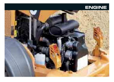
The 721E and 821E are powered by a Tier III Case 667TA/EED diesel. This electronically-controlled 6.7 litre engine provides a choice of three power and torque ratings, designed to perfectly match the requirements of the machine in any application, maximising fuel economy.
