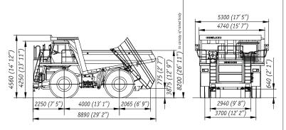
\*Overall dimensions are specified for basic kitting-up of the dump truck
