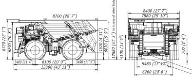
\*Overall dimensions are specified for truck with standard option
