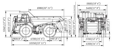
\*Overall dimensions are specified for basic kitting-up of the dump truck
