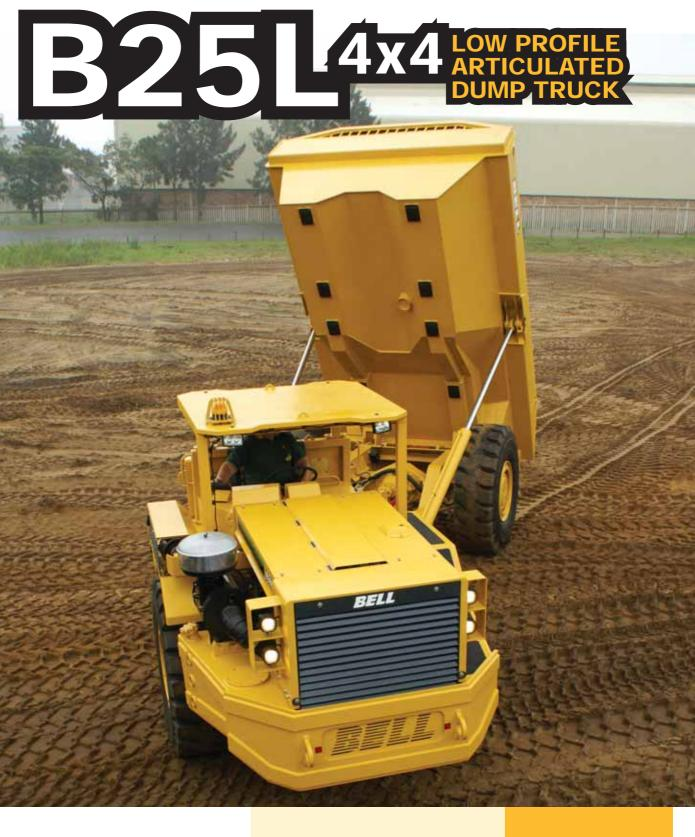
Gross Power: 205 kW (275 hp) Gross Torque: 1 100 Nm (810 lbft) Rated Payload: 23 000 kg (50 600 lbs)
