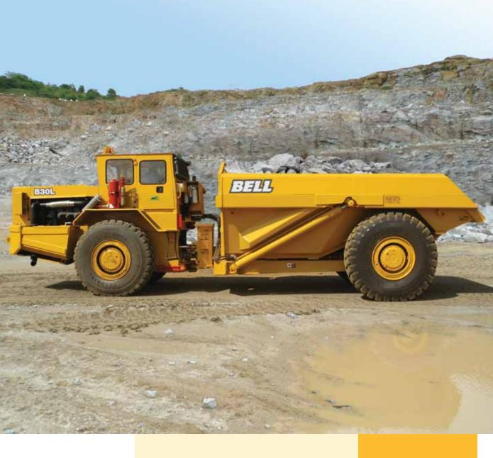
Gross Power: 230 kW (308 hp) Gross Torque: 1 295 Nm (955 lbft) Rated Payload: 27 000 kg (59 524 lbs)
