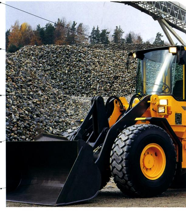
A Volvo six-cylinder engine and TP Linkage put power behind the world's widest range of attachments
