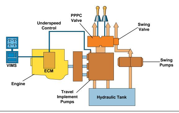
Exclusive Caterpillar Proportional Priority Pressure Compensating (PPPC) valves are used in both the front structure and travel systems.
