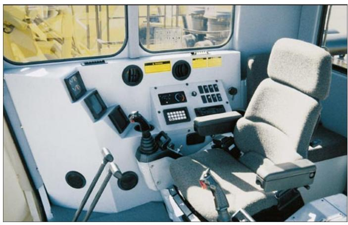
Spacious operator compartment measures 1790 mm (5'10") wide by 2178 mm (7'2") long by 2236 mm (7'4") high.
