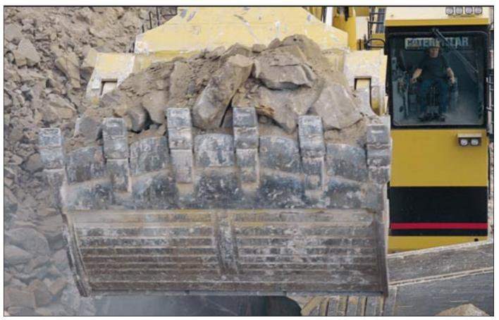
High fill factors for the 5230 Front Shovel and Mass Excavator set this machine apart from the competition. Caterpillar's quality design improves breakout and crowd forces, increasing fill factors.
