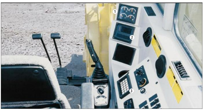
The VIMS system continuously displays critical machine data. This information can be used to keep the 5230 performing at top production levels.
