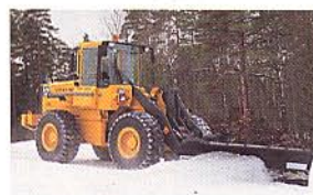
Snow blade For snow clearance. Hydraulically adjustable.
