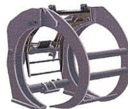
Heel/kick-out For holding a single log and making higher stacks. Requires 4th hydraulic control.
