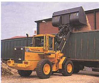
High-dump wood chip bucket. Volume 3,6-13,0 m 3 .
