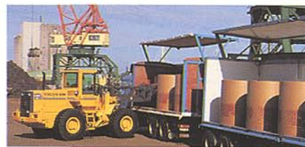
Hydraulic bale clamps can handle everything from waste paper bales to finished reels of recycled paper.
