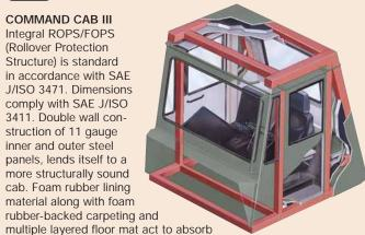
sound and control interior temperature. A properly maintained cab from Euclid, tested with doors and windows closed per work cycle procedures in SAE J1166, results in an operator sound exposure Leg (Equivalent Sound Level) of 79 dB(A). A three-point rubber isomount arrangement to the deck surface minimizes vibration to the operator compartment.
