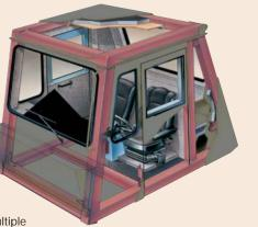
layered floor mat act to absorb sound and control interior temperature. A properly maintained cab from Hitachi, tested with doors and windows closed per work cycle procedures in SAE J1166, results in an operator sound exposure Leg (Equivalent Sound Level) of 81 dB(A). A three-point rubber iso-mount arrangement to the deck surface minimizes vibration to the operator compartment.
