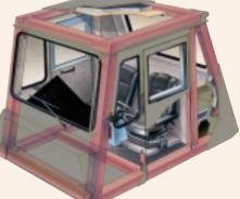
layered floor mat act to absorb sound and control interior temperature. A properly maintained cab from Euclid, tested with doors and windows closed per work cycle procedures in SAE J1166, results in an operator sound exposure Leg (Equivalent Sound Level) of 81 dB(A). A three-point rubber iso-mount arrangement to the deck surface minimizes vibration to the operator compartment.
