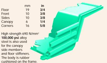
The Euclid horizontal stiffener design minimizes stress concentrations, by dissipating load shocks over the entire body length. Closely spaced stiffeners provide additional protection by minimizing distances between unsupported areas.
