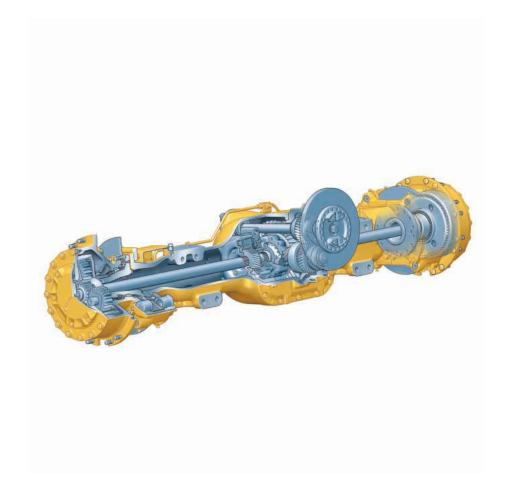
**Parking Brake.** The parking brake has been moved from the transmission to the center axle. This new design delivers higher heat capacity and abuse resistance.
