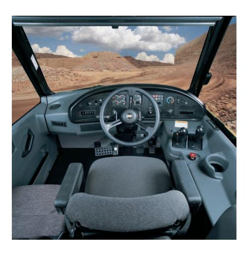
**Transmission and Hoist Levers.** The hoist lever has been redesigned and relocated to provide easy and comfortable operation. The transmission lever continues to offer excellent comfort along with controls for top gear limit, transmission hold and neutral lock.
