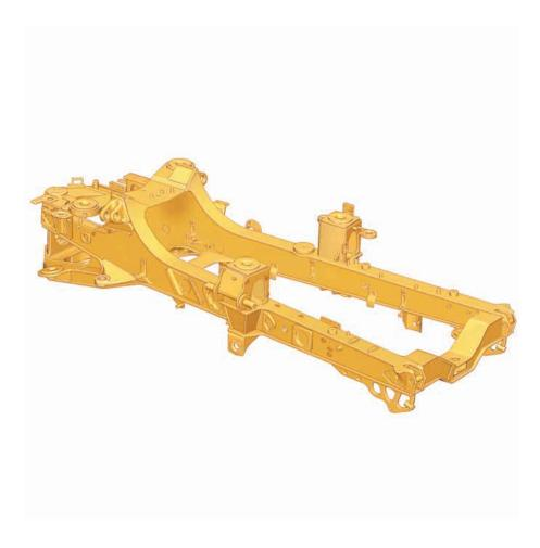
Front Frame. The front frame design features a large box-section, and wide, stiff frame beams to handle torque loads. The divergent frame design decreases stress in the hitch area and optimizes suspension geometry. The frame has been designed to make maximum use of robotic welding for increased durability.
